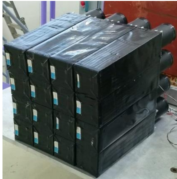
Figure 13: Stack of lead crystal calorimeters.
