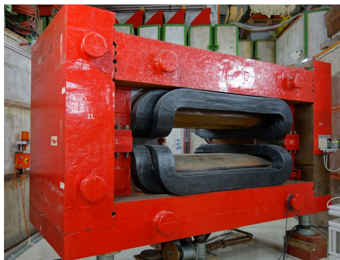
Figure 14: BRM, 1.35 T dipole magnet
