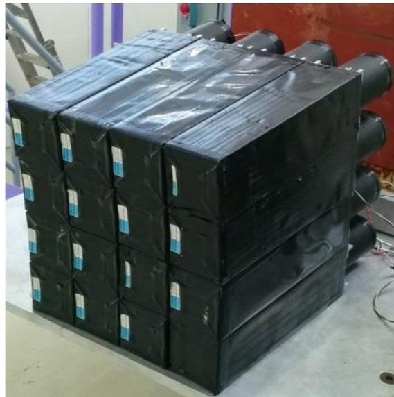
Figure 7: Stack of lead crystal calorimeters.
