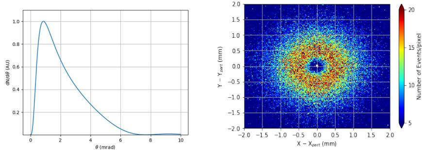
Figure 4: Left panel: Theoretical angular distribution of TR X-rays from a single foil. Right panel: MIMOSA chip simulated output. The relative positions of TR pixel (X-Y view) with respect the electron one are shown. The color scale indicates the number of events detected in each pixel. The white hole in the middle of the image shows the  $4 \times 4$  masked pixels corresponding to the electron positions.
