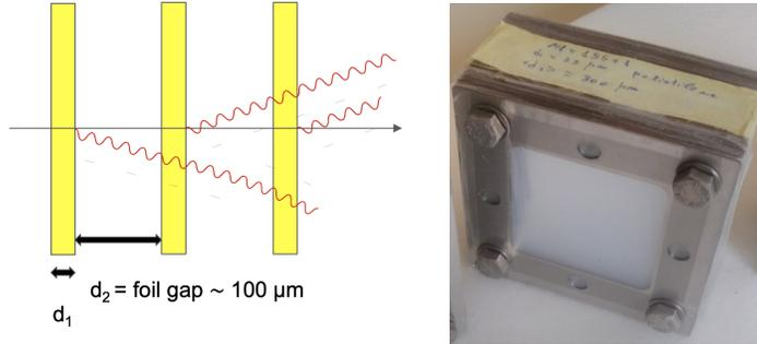
Figure 3: Left panel: Sketch of a multilayer radiator. Right panel: radiator module made of 155 polyethylene foils  $25 \mu\text{m}$  thick and  $300 \mu\text{m}$  of gap.
