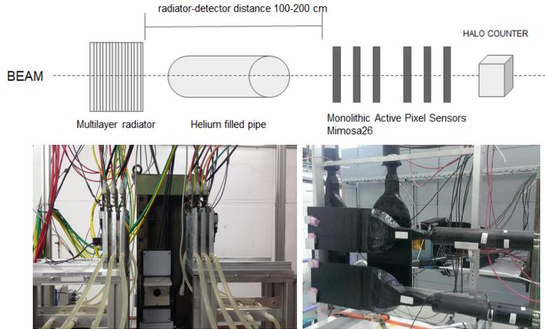
Figure 2: Top panel: Scheme of the experimental setup. The beam direction correspond to z-axis of the reference frame. Bottom left panel: Mimosa telescope. Bottom right panel: Halo counter.
