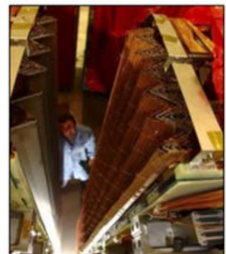
The image shows the steel absorber used in the calorimeter of the ATLAS experiment
