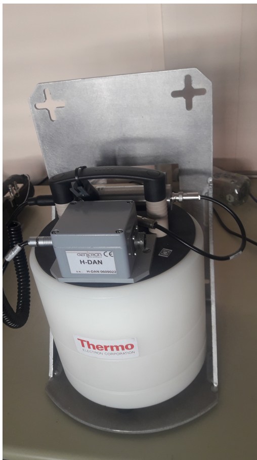
Figure 13: WENDI Neutron detector.
