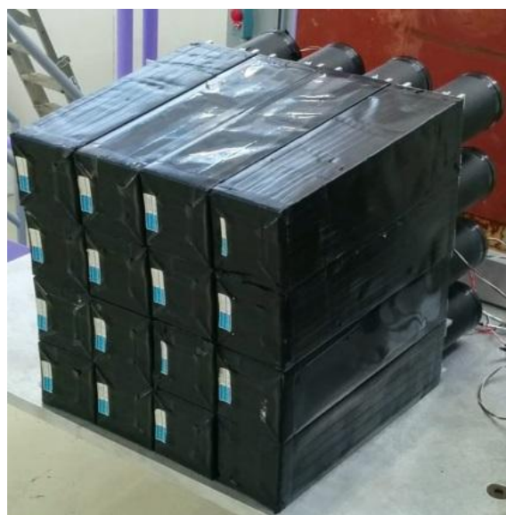
Figure 16: Stack of lead crystal calorimeters.
