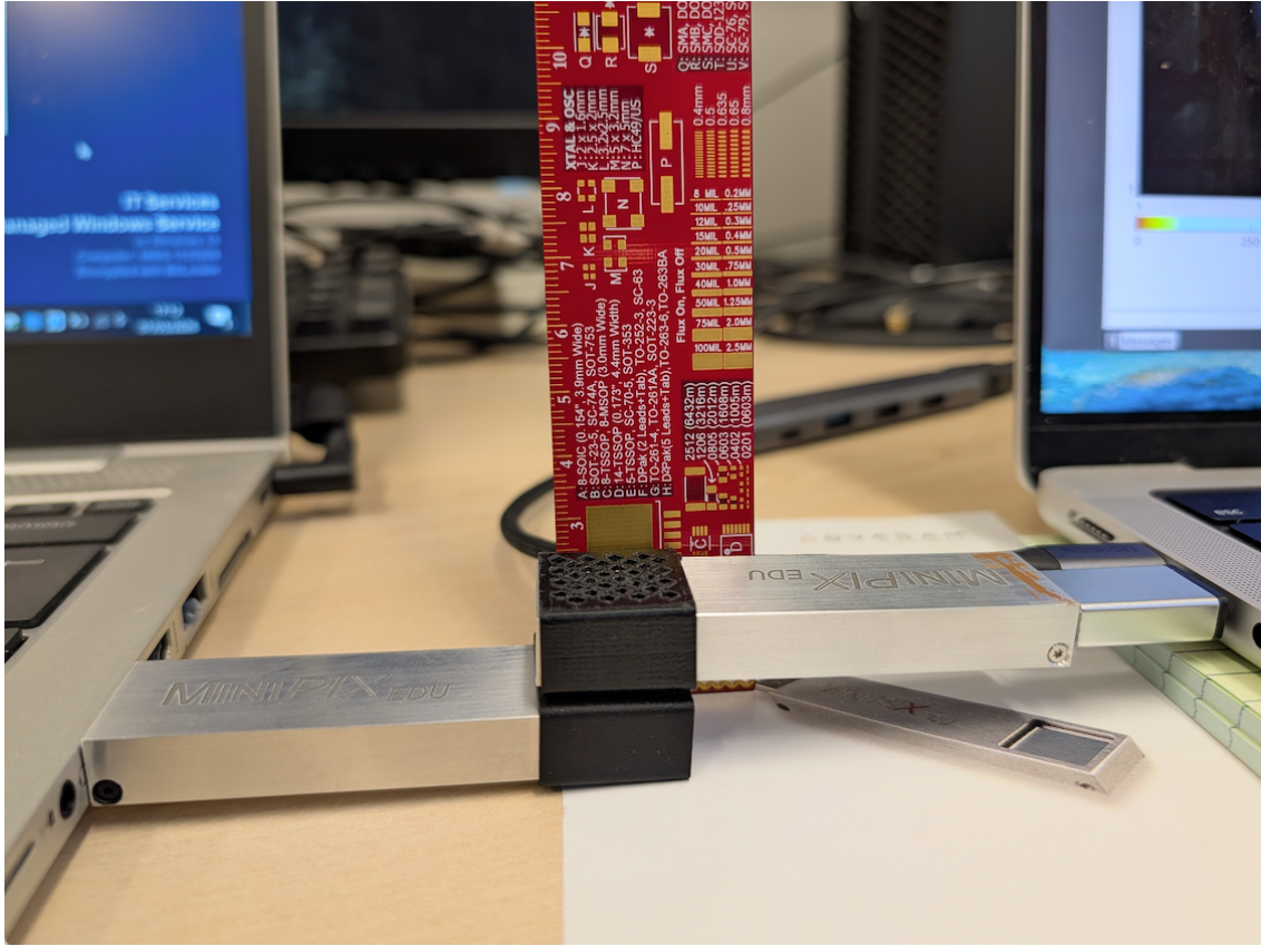
Figure 5: The setup we used to try and identify a cosmic muon that travelled perpendicular to the detectors
